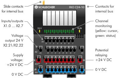
The RIO C24-10 expert module provides up to 4 mutually independent up/down counters. They count clock pulse signals. Other inputs can be used to control counting, alter the counting direction and reset the counter. The counter value is compared with up to two thresholds. If the value exceeds or falls below the threshold the outputs switch.
